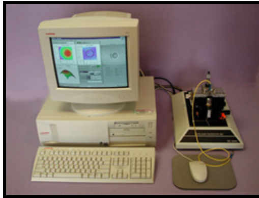
Interferometer Measuring a Singlemode Connector
